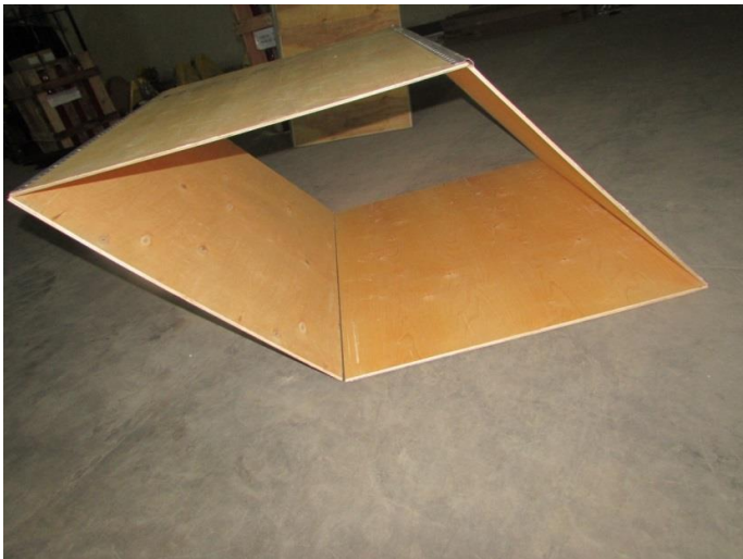
COLLAPSED CONDITION OF SIDE COVER (indicative fig)
